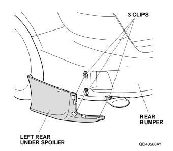
9. While applying light pressure against the left rear under spoiler, carefully remove the adhesive backings.
