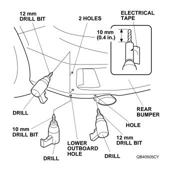
5. Install one clip into each 12 mm hole in the direction shown. Push in each clip until you hear it "click," then check to make sure the clips are secure in the rear bumper.
